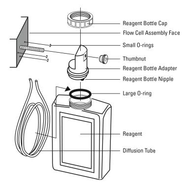
Figure 21: Reagent Bottle Assembly
