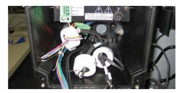
Figure 11: Ferrite Installation
