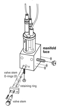
Figure 22: Flow Cell Assembly
