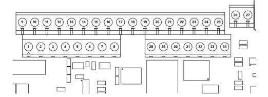
**Figure 9: Terminal Assignments**
