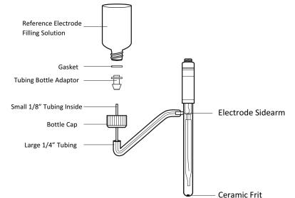
Figure 13: Reference Electrode with Filling Solution
