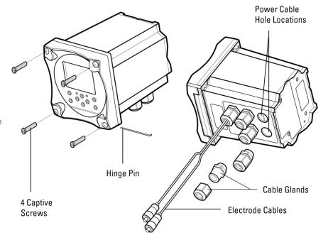
Figure 7: Electronics Enclosure with Cable Glands
