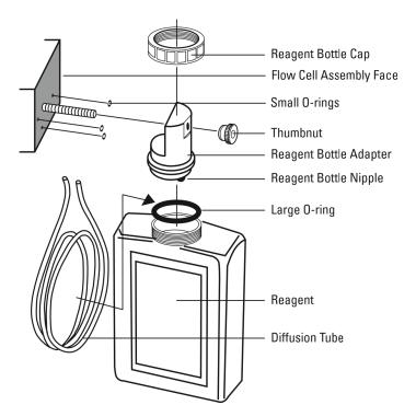
Figure 10: Reagent Bottle Assembly
